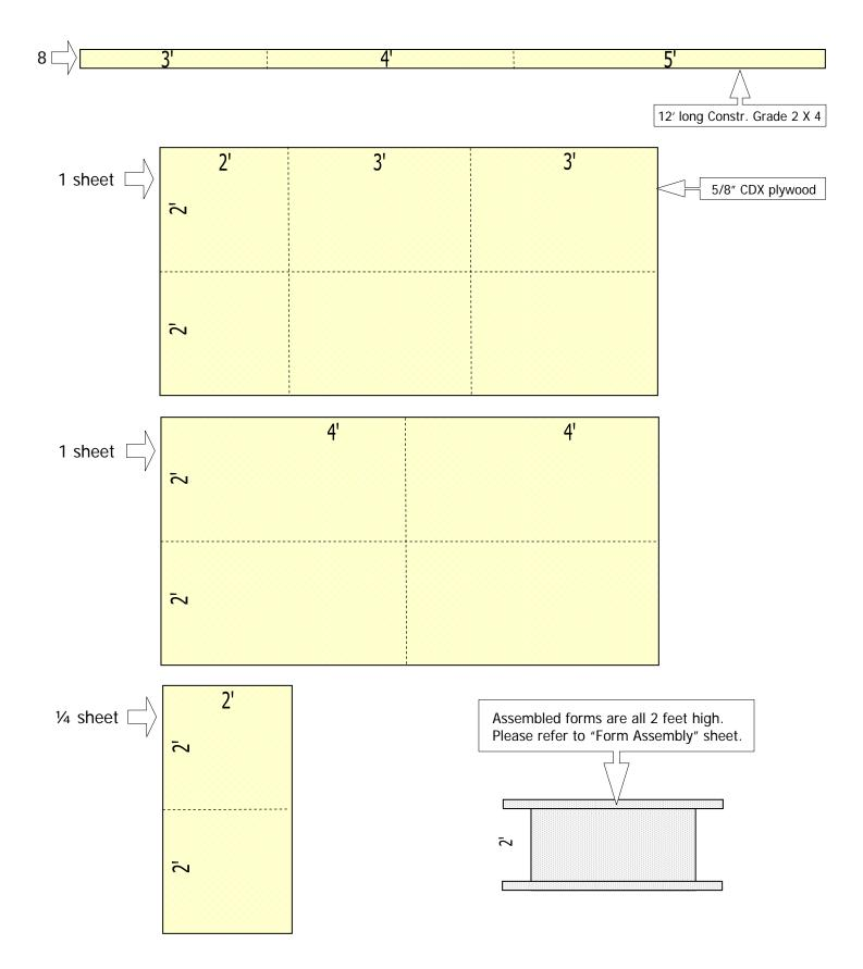
Cut 2X4 (stringer) a minimum of 1' longer than the panel, i.e., for a 3' panel use 4' stringers. Minimum 6" overhang on both ends.
